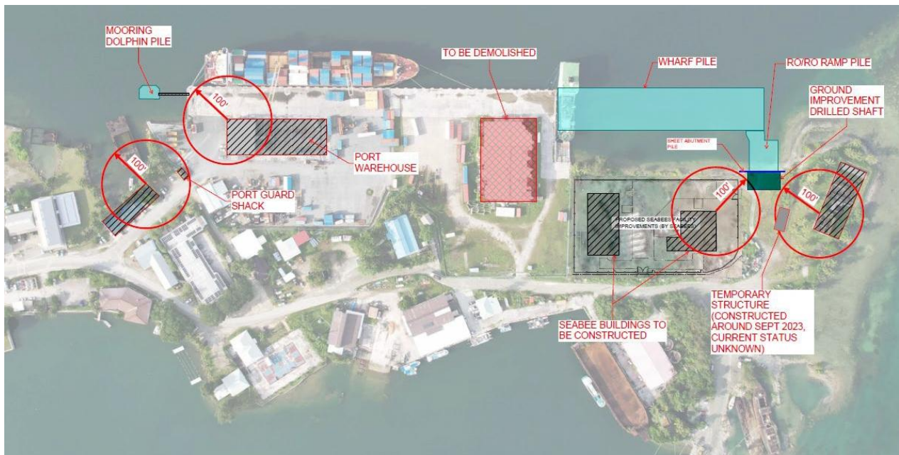
Figure 12: Seaport Construction Activity Areas
